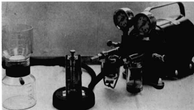
Figure 1—Vacuum system used in the air sampling techniques.
